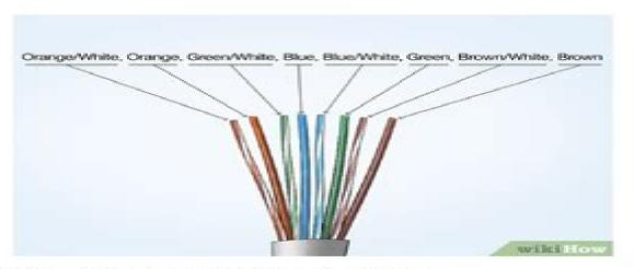
Step 1: Strip the cable jacket about 1.5 inch down from the end.
