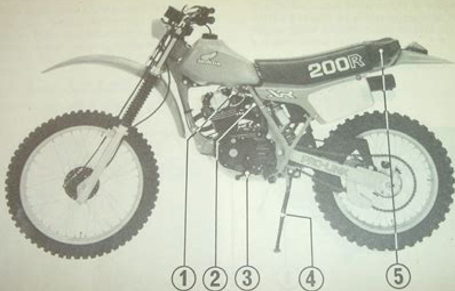
(1) Fuel valve (2) Choke lever (3) Gearshift pedal (4) Side stand (5) Tool bag
