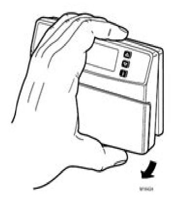
If you insert new batteries within 20 to 30 seconds of removing the old batteries, the system retains the current time and day. If the display is blank, the batteries are dead or installed incorrectly. You must reset the time and day. Refer to Setting the Clock section for instructions.
