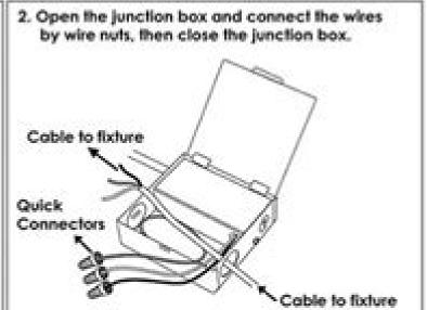
3. Connect the fixture with the junction box using the twist connector, place the junction box into the ceiling or fix it on the joist.
