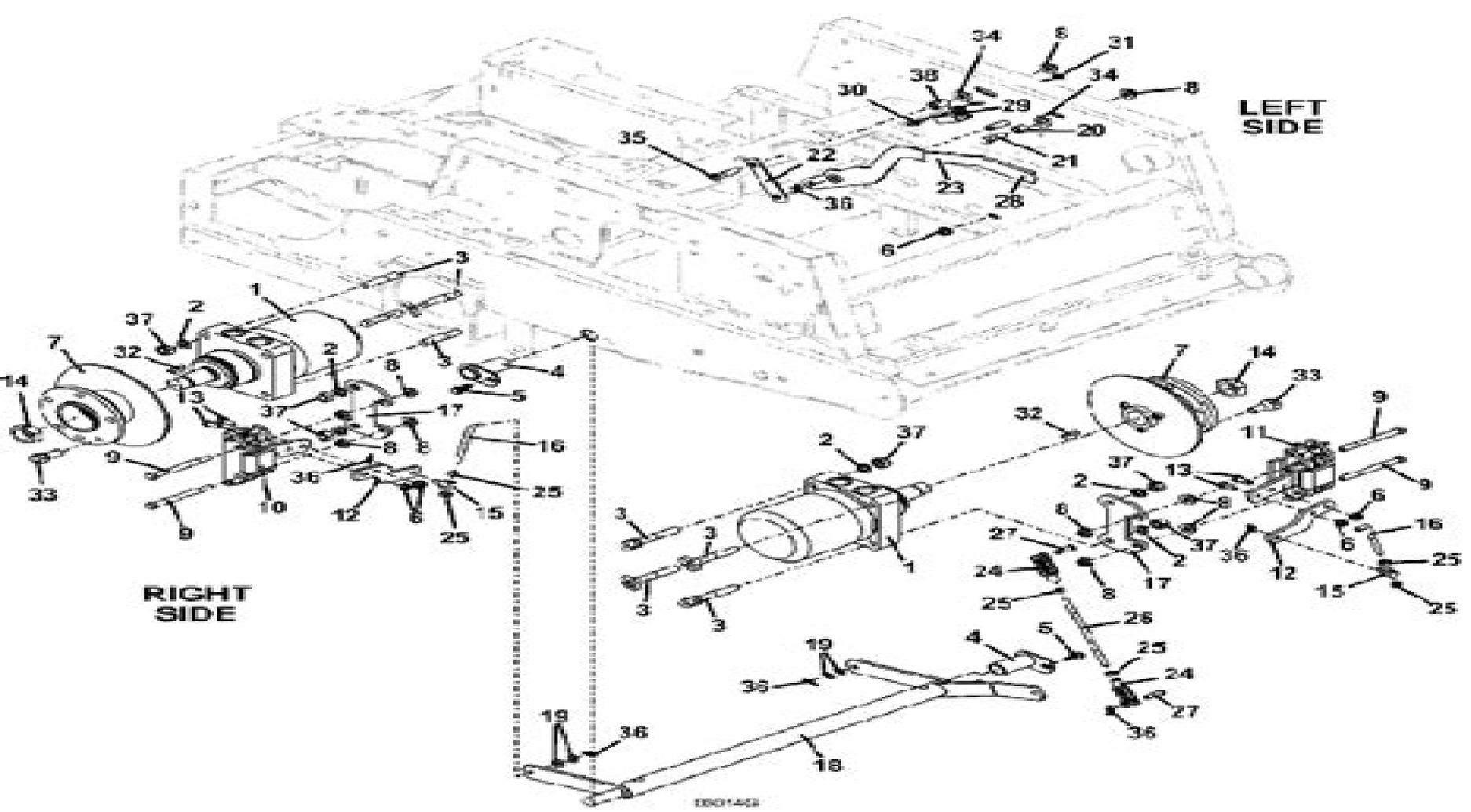
Wheel Motor & Brake Assembly
