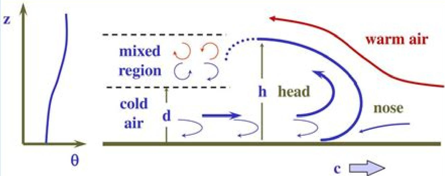
Schematic diagram of a steady gravity current
