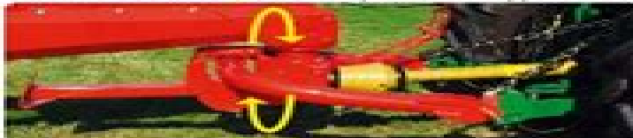
The Gyrodine swivel hitch: 540 or 1000 min -1
