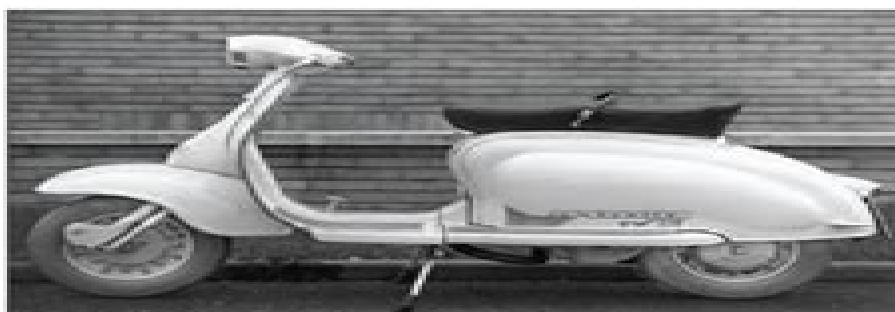
The TV175 S2 was an excellent scooter, but not without problems in the beginning. The frames on the first batch were weak and had to be cut apart and strengthened with vertical ribs welded in along the rear half of the main tube. These examples are commonly known as 'ridgebacks'.
