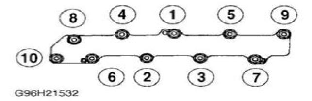
Fig. 3: Exhaust Manifold Tightening Sequence Courtesy of GENERAL MOTORS CORP.
