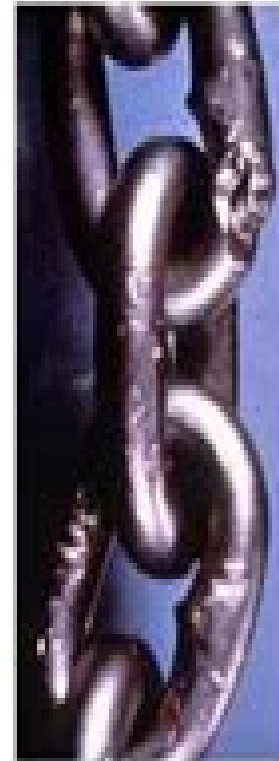
HEAT DAMAGE & NICKS AND GOUGES
