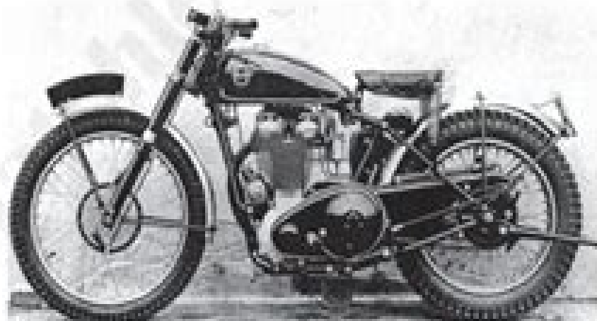
A reader's definitive photograph (the courtesy of Matchless Special for the 1955 100cc Matchless, 100cc shown here in trade gear with hydraulic motor, pre-1955 carburettor, rigid frame, Barman box and the left-side of forward-mounted magneto (introduced June/September 1955). The Lucas magneto here is of course the 'Walter' type. It has the wire-type from Brake brought in September 1955; the full-size from last year arriving until 12 months later.
