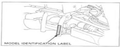
The model identification label is located on the left side frame down tube.
