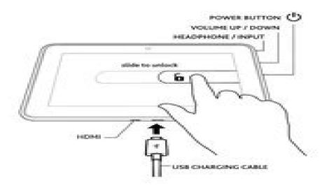
To charge your Kindle, connect it to the USB charging cable as shown. Connect the opposite end of the USB charging cable to a Kindle PowerFast accelerated charging accessory (sold separately), or other USB power adapter. To learn more about charging accessories, visit www.kindle.com/support/charging.
