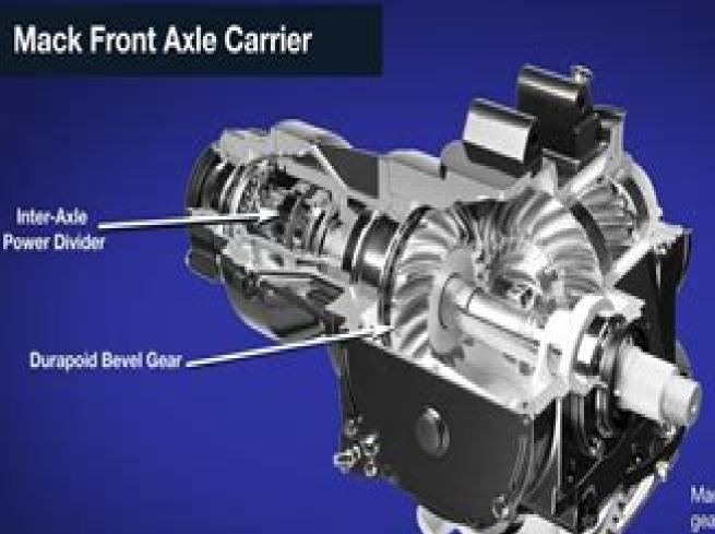
Mack's patented Durapoid bevel gear design eliminates localized stress and tooth-end loading to improve fuel economy, maximize energy efficiency and extend gear life.
