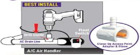
CLOSED DRAIN LINE - Using the provided Drill Guide, drill a hole into the drain line as close to the air handler as possible. Then attach accesspoint adapter.
