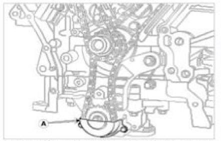
Remove the oil pump chain tensioner assembly (A)
