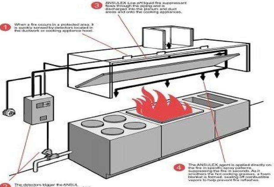
The detectors trigger the ANSUL AUTOBAN's release mechanism which actuates the system... prescuriting the agent storage tank and automatically shutting of appliance energy sources in the event of a fire.
