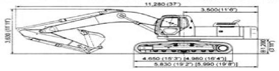
2.3 6.50m (21"4") Boom+4.15m (13"7") Long Arm+1.20m3 (1.57cu-yd) Bucket+600mm (24") Shoe
