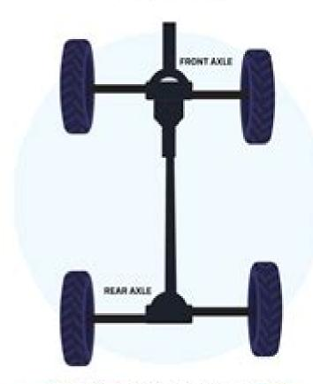
AWD sends power to either the front axle or rear axle in normal driving conditions. If the vehicle detects a lack of traction it will engage to all wheels.
