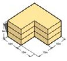
Heated Floor Area (A, 2\*: 675 m/r Envelope Area (A\_3: 1,300 mg **Volume (V)**: 2,700 mil Heat Loss Form Factor(A,/A, ) 1.94 terface to Volume ButleCA\_AVE B.48 t/re
