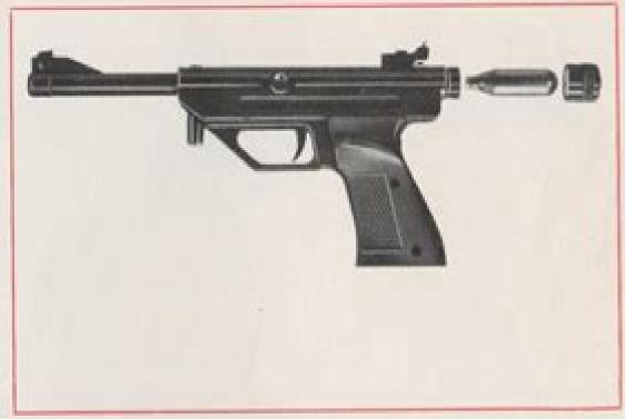
The locking cap can be removed only when all the carbon dioxide has been allowed to escape from the pressure chamber. The residual CO<sub>2</sub> can be released by forcing the cocking knobs firmly back towards the locking cap whilst the pistol is NOT cocked. Never use any force when removing the locking cap, and NEVER use any tools, e.g., grips, pipe wrench, et altera to un-screw this cap!
