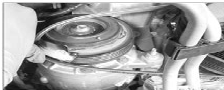
12.13 Install the belt installation tool and rotate the crankshaft pulley until the belt is lifted onto the pulley
