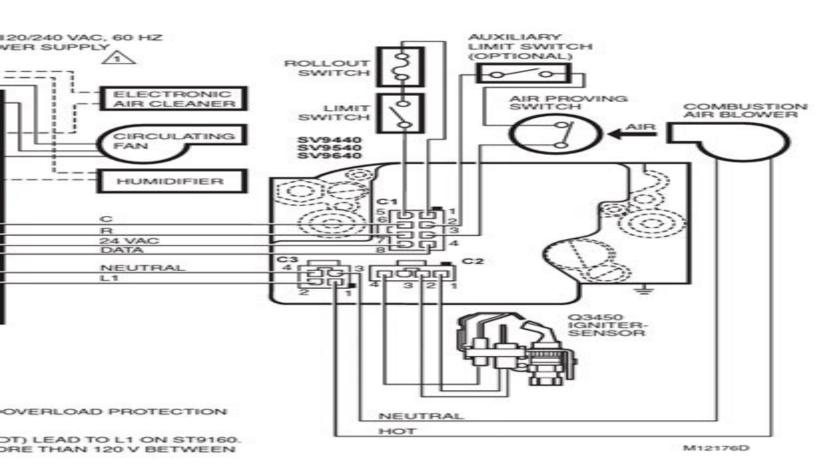
assisted warm air furnace with ST9160 Electronic Fan Timer.
