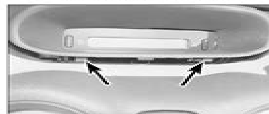
27.2b ... to compress the internal plastic retaining tabs (arrowed)
