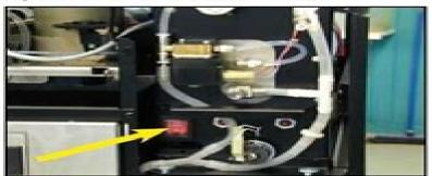
Turn main TS module power switch to the \_ON\* position.
