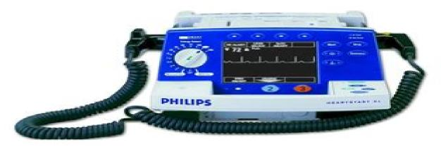
Philips Medical Systems' M4735A HeartStart XL offers advanced and basic life-support clinicians a compact. lightweight, easy-to-use defibrillator/monitor with both Manual and AED capabilities. HeartStart XL features Philips' patented SMART Biphasic waveform, ECG monitoring, synchronized cardioversion, and optional noninvasive pacing and SpO<sub>2</sub>.
