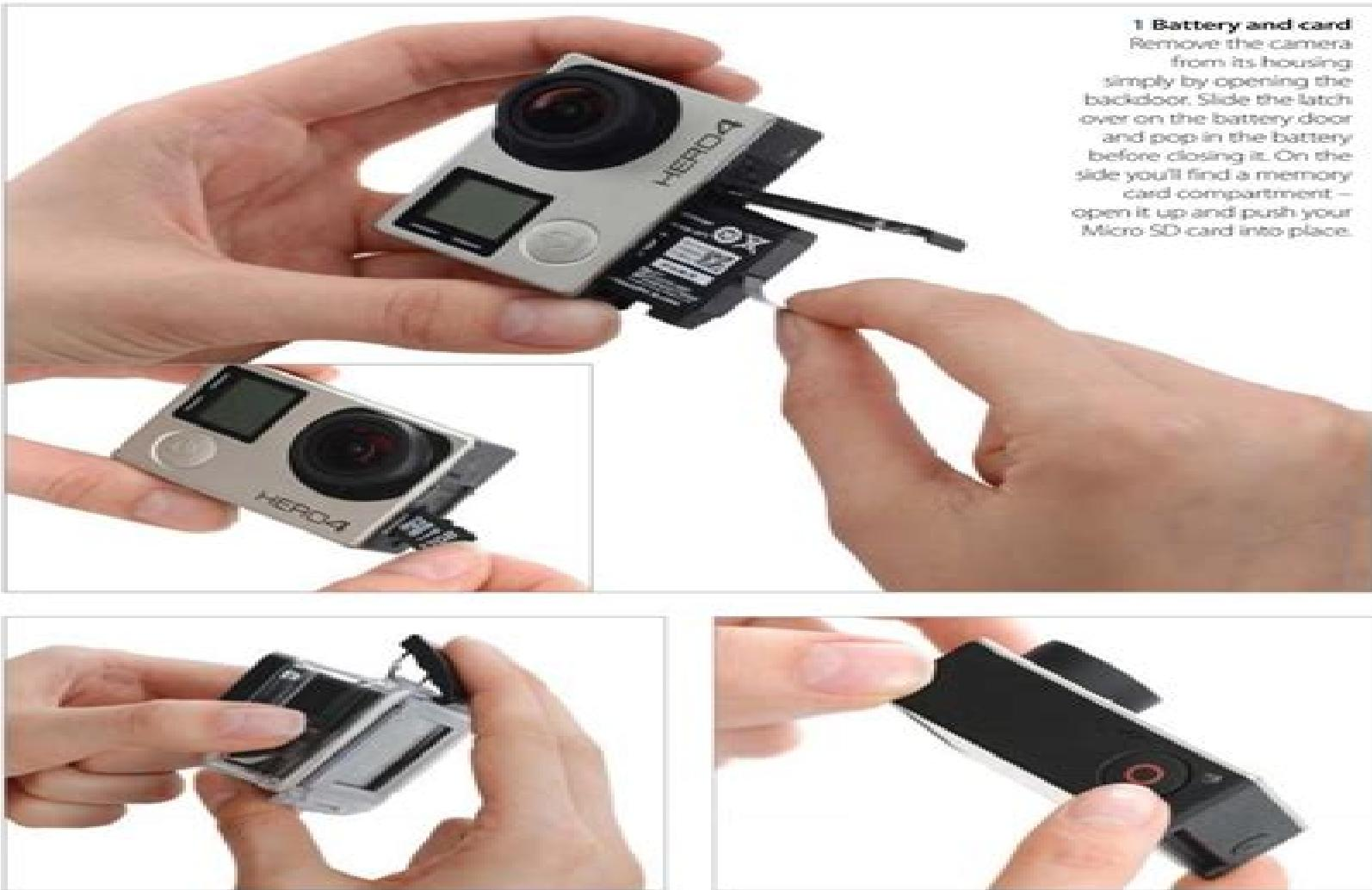
**2 Rehouse:** It's important that you put the housing back on your camera correctly to ensure it's kept waterproof and safe from dust and debris. So slide the camera back into its housing and close the backdoor by snapping the top latch down firmly.
