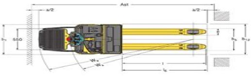
Ast =  $W_a$  + x +  $I_6$  + a (see lines 4.33 & 4.34): a = Minimum operating clearance (VD.), standard = 200 mm. BITA recommendation = 300 mm):  $I_6$  = Load length
