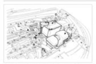
Disconnect the ECM connector and then remove the EC
