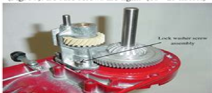
Fig. 59 Secure the three lock washer screw assemblies into the bottom cover.
