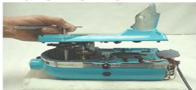
Fig. 60 Initial mating of bottom cover to gearcase - motor housing.
