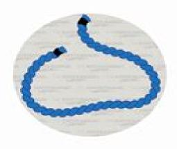
Form a small loop leaving enough rope for the desired loop size.
