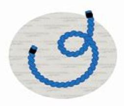
Form a small loop leaving enough rope for the desired loop size.
