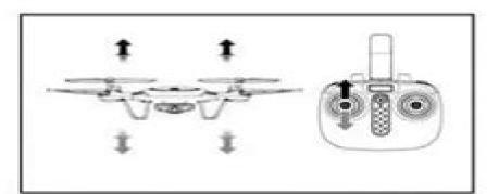
When the left joystick (Accelerator) is pushed upwards or downwards, the aircraft will ascend or descend correspondingly.
