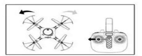
When the left joystick (Accelerator) is pushed towards the left or right, the aircraft will turn left or right correspondingly.
