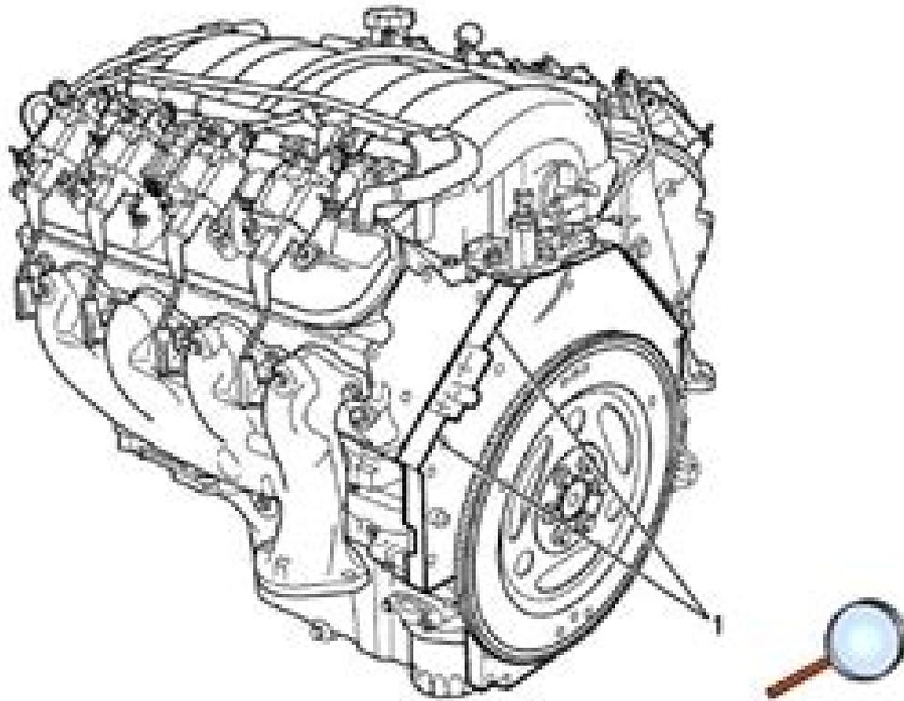
The vehicle identification number (VIN) (1) is located on the left side rear of the engine block and is typically a 9 digit number stamped or laser-etched onto the engine at the vehicle assembly plant.
