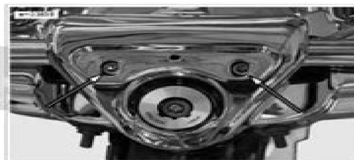
Figure 2-91. Loosen Upper Handlebar Clamp Screws (FLHR/C)
