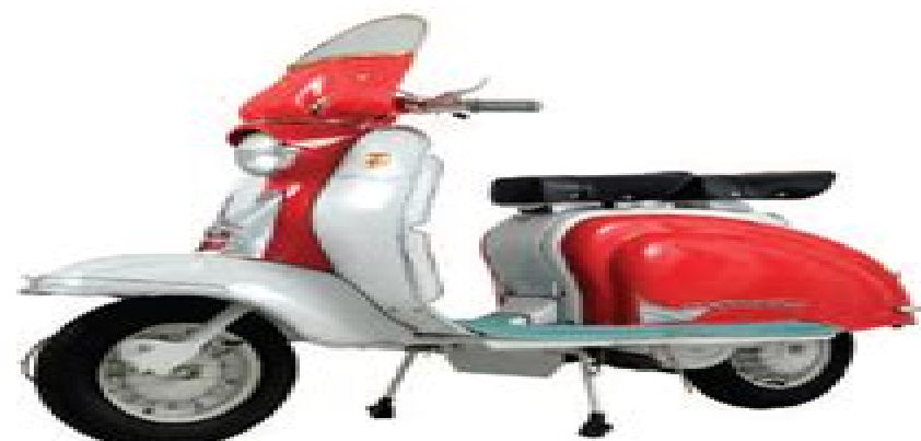
An Innocenti factory photograph of a very early LI150 Series 1 as denoted by the vertical slots at the front of the side panels which were soon abandoned.
