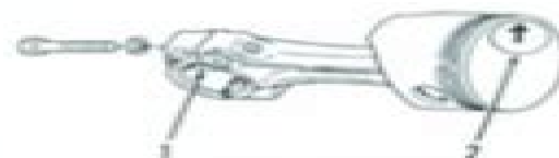
Fig. K109—Assemble piston to connecting rod so arrow mark (2) on piston crown is aligned with machined surface (1) on connecting rod and cap.
