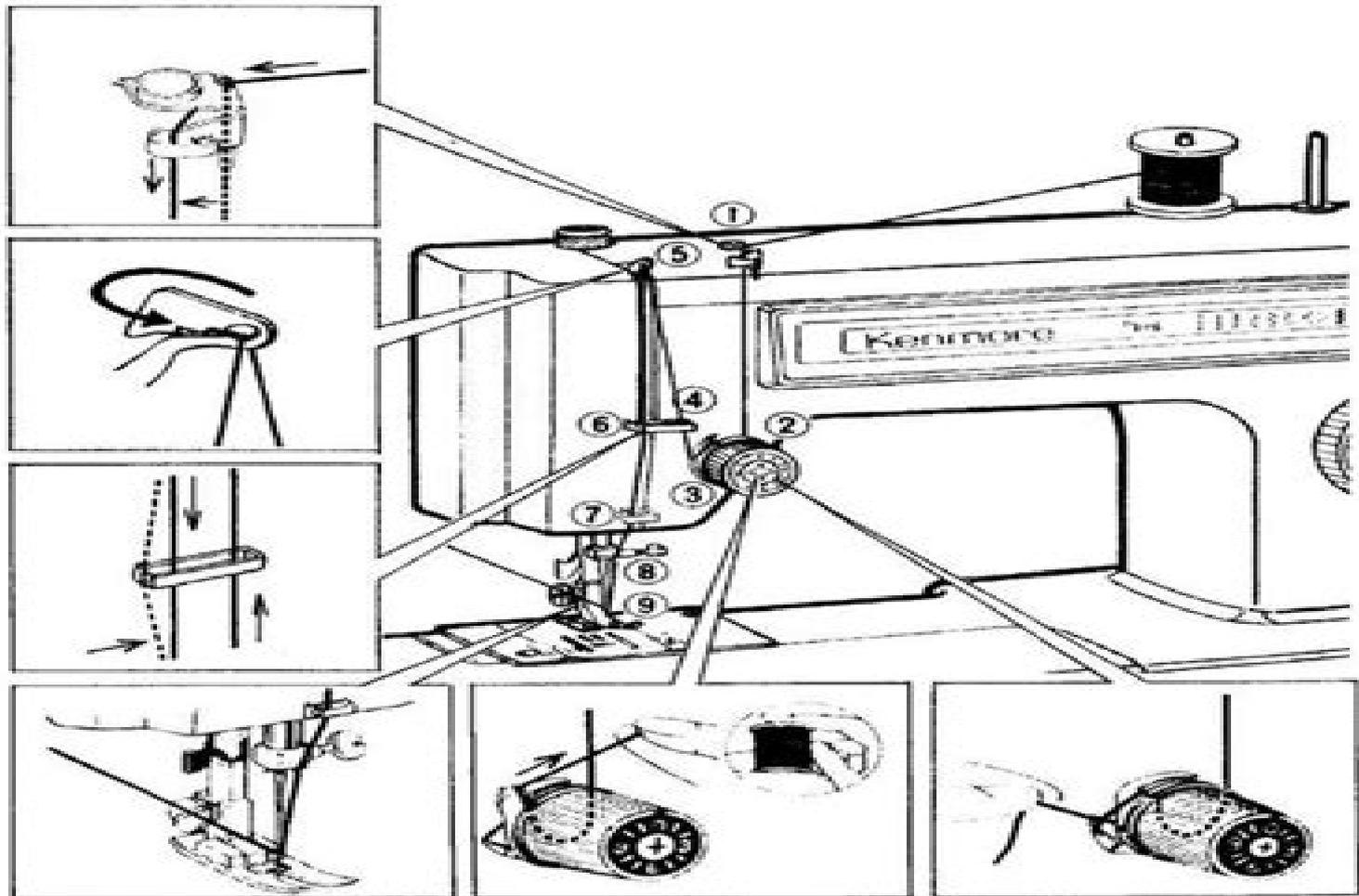
1. Raise thread take-up lever to its highest position by turning hand wheel toward you. Raise presser foot lever. Place thread spool on spool pin. Draw thread through thread guide 1. Holding spool stationary with right hand, pull thread through the tension discs. Pull the end of the thread taut with the left hand.
