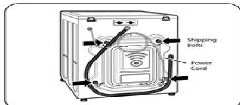
1. Starting with the bottom two shipping bolts, use the wrench (included) to fully loosen all four shipping bolts by turning them counterclockwise.
