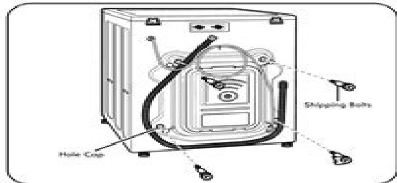
2. Remove the bolt assemblies by wiggling them slightly while pulling.
