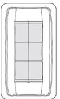
The foam pad attaches to the backside of the backrest leather and protects the leather from excessive wear.
