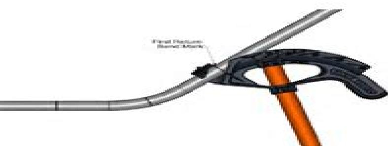
*Note: Some over bending may be required to allow for spring back of the conduit. The resting condition of the conduit is to be at the final angle desired.*
