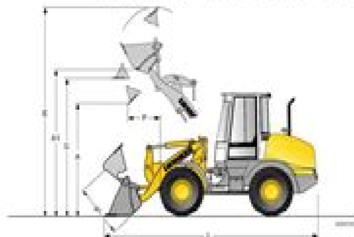
Fig. 20: Attachment – 4 in 1 bucket
