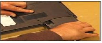
To begin the disassembly procedure, make sure the unit is powered off. Remove the battery.
