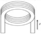
A 25.0 cm solenoid has 1800 loops and a diameter of 3.00 cm. Calculate the magnetic field in the air core of the solenoid when a current of 1.25 A is flowing.
