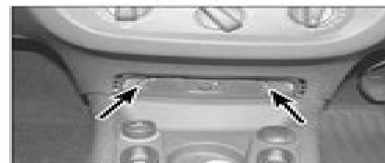
26.4b ... and undo the two screws (arrowed) now exposed
