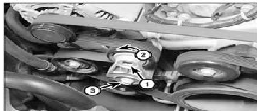
12.6a V6 engine accessory drivebelt tensioner details
