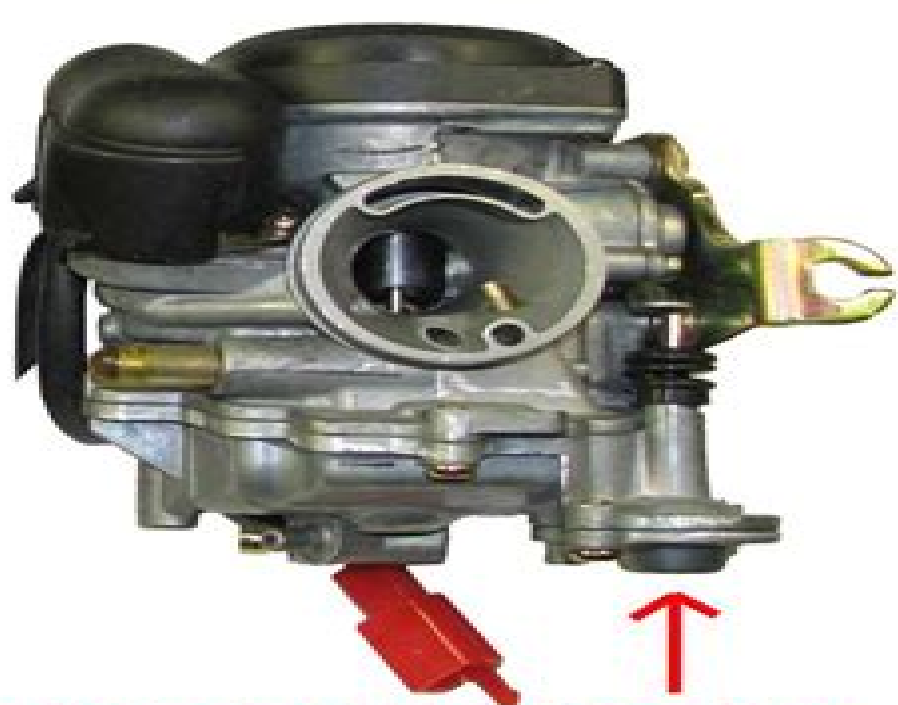
GY6 50cc Carb With Build-in Fuel Pump
