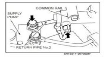
(10) Replace old gaskets with new ones. Connect the return pipe No.2 to the supply pump and the common rail, and tighten two union bolts.
