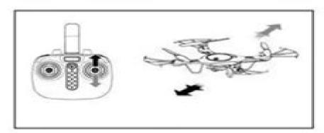
When the right joystick (Turning Rudder) is pushed upwards or downwards, the aircraft will advance forward or backward correspondingly.
