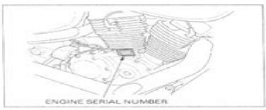
The engine serial number is stamped on the right crankcase below the rear cylinder.
