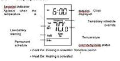
. When Cool On is flighting this means the compressor protection is engaged (see
